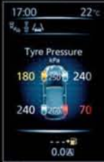
TYRE PRESSURE MONITORING SYSTEM No more guesswork: Each tyre pressure is displayed on screen and a signal lights up on the dash if the pressure is low.
